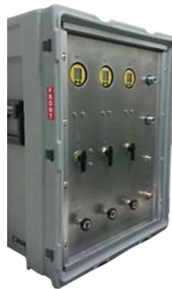
Pneumatic Test Platform
